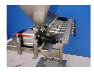
For less fluid fillings the unit can be supplied with a turn shaft, which creates a vacuum in the chamber assisting the refilling of the chamber between strokes.
